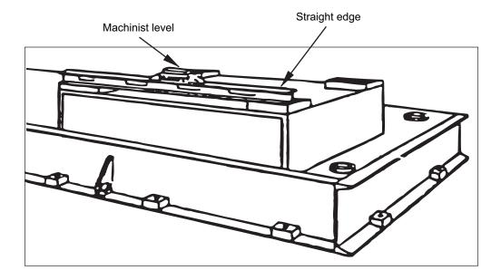
Figure E.9—Leveling Driver End Lengthwise (Typical)
