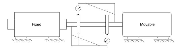
Figure D.1—Reverse Rim (Dial) Alignment
