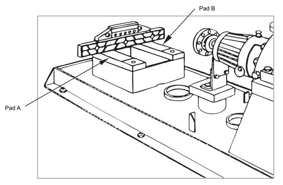
Figure E.3—Leveling Driver End Crosswise
