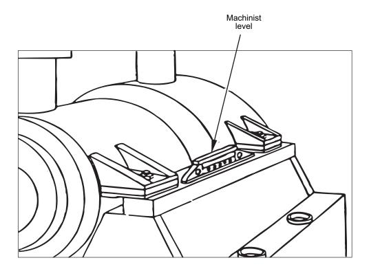
Figure E.10—Leveling Pump End Lengthwise
