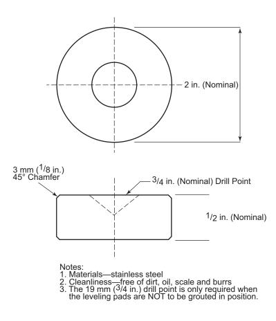
Figure H.1—Typical Mounting Plate Leveling Pads
