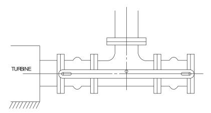
Figure C.3—Exhaust Piping Expansion Joint Application Utilizing Tie Rods
