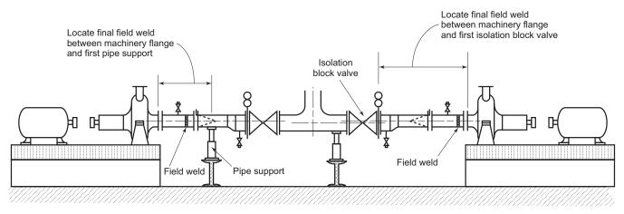
Figure B.5—Final Field Weld Location
