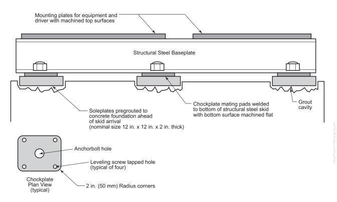
Figure D.1—Typical Mounting Plate Arrangement for Baseplate Mounted Special-purpose Equipment
