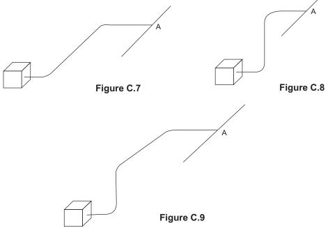
the specified limits. Figure C.7 through Figure C.9 apply to inlet piping as well as exhaust lines, except that the takeoff from a steam header should be on the top.
