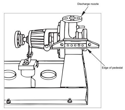
Figure E.5—Leveling Pump End Lengthwise
