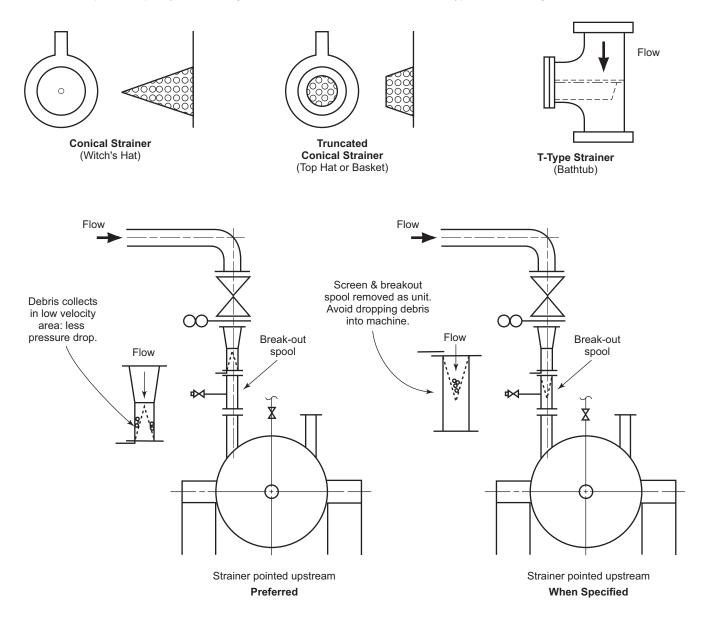
2.8.2.8 The point of the conical strainer shall face upstream in the piping. Screens in T-type strainers shall point with the flow.
