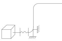
Figure C.14—Improper Use of Spring Support on Piping Expansion Joint
