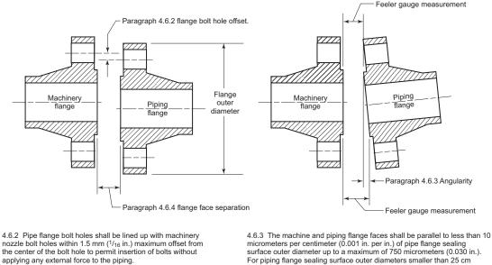
4.6.4 Flange face separation shall be within the gasket spacing plus or minus 1.5 mm ( $^{1}_{16}$  in.). Only one gasket per flanged connection shall be used.
