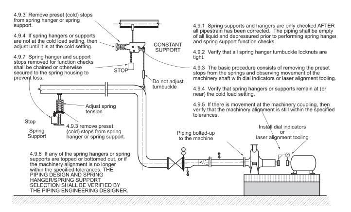
Figure B.8—Spring Hanger Function Checks
