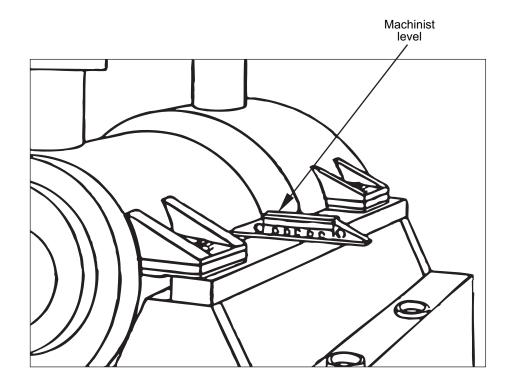
Figure E.7—Leveling Pump End Crosswise
