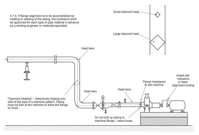
Figure D.3—Diamond Heating Pipestrain Relief
