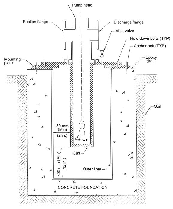
NOTE Can = Pressure Retaining Casing
