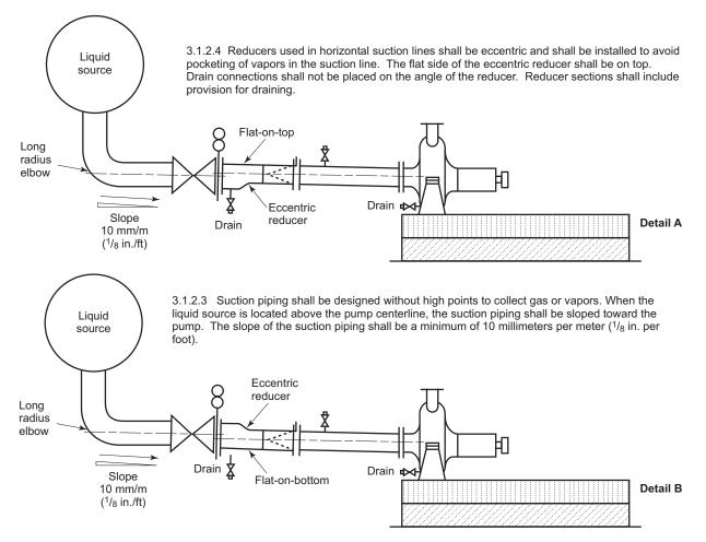
3.1.2.4 Note 2: When the piping must be completely drained to remove hazardous liquid or solids before performing maintenance, the eccentric reducer in the horizontal pump suction line may be oriented with the flat side on the bottom. For example, it is desirable that hydroflouric acid piping be completely drained to avoid pockets of material that may prove hazardous to maintenance personnel.
