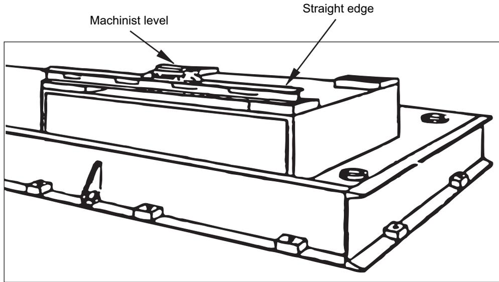
Figure E.9—Leveling Driver End Lengthwise (Typical)
