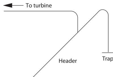
**Figure C.11—Recommended Turbine Inlet Piping Arrangement at Header End with Drop Leg**
