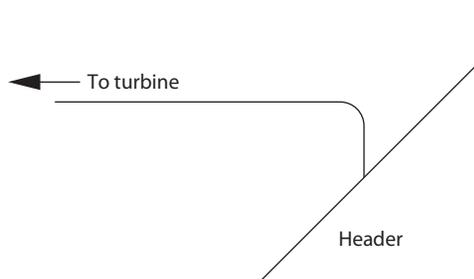
**Figure C.10—Recommended Turbine Inlet Piping Arrangement from Header**
