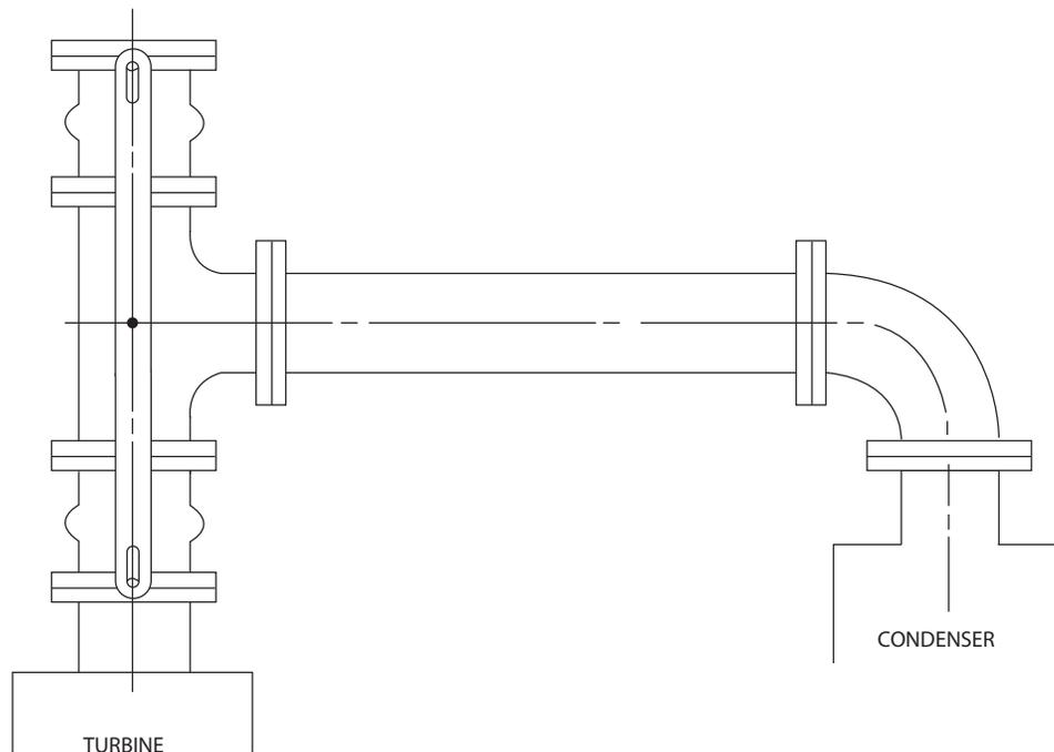
**Figure C.4—Condensing Turbine Expansion Joint with “UP” Exhaust**
