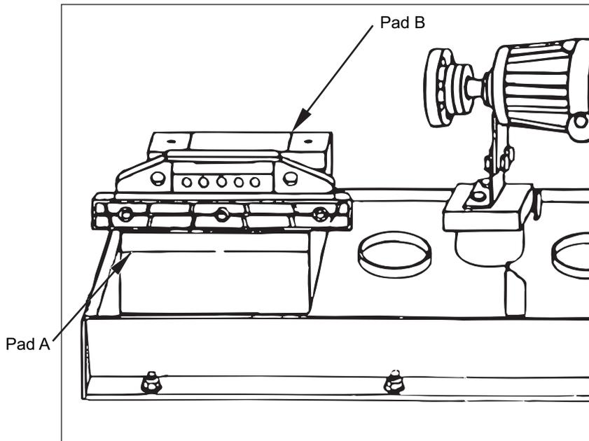
Figure E.4—Leveling Driver End Lengthwise
