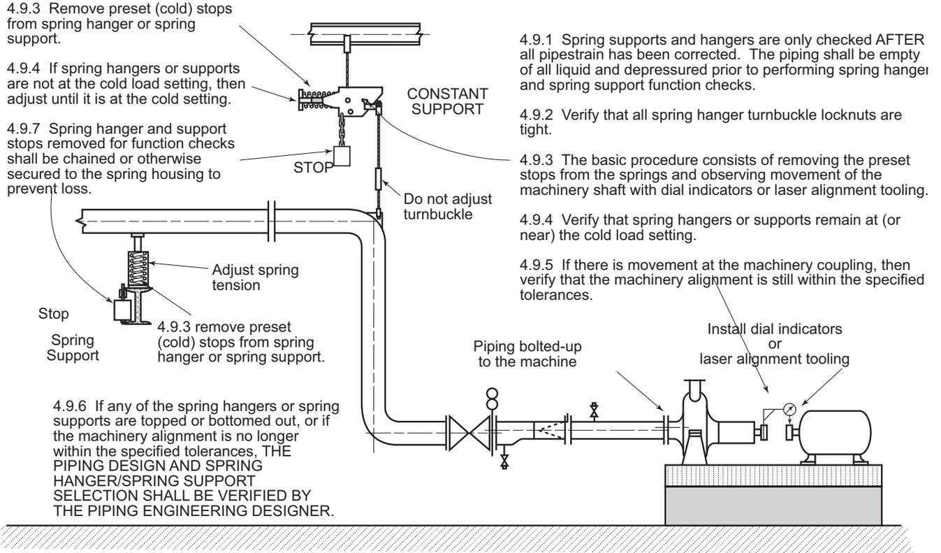
**Figure B.8—Spring Hanger Function Checks**
