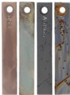
Corrosion Coupon Analysis
